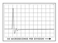
Fig 3. Impulse Response (Typical) of TC25
