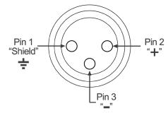
Fig 1. XLR Output Connector Assignment of TC25
