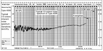
Fig. 10. Typical third-octave inherent-noise spectrum of Type 4006.
