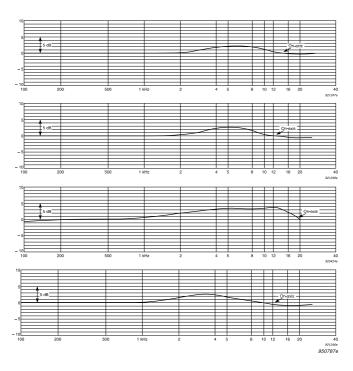
Fig. 11. Response characteristics of APE L30B (top), APE L40B, APE L50B and APE L110C.
