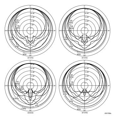
Fig. 12. Directional characteristics of APE L30B (top left), APE L40B, (top right), APE L50B and APE L110C.
