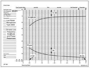
Fig. 9. On-axis low frequency amplitude and phase response of Types 4003 and 4006.
