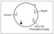
Fig. 1. External view of the output socket of the Type 4003.
