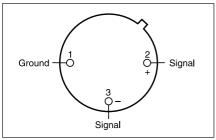
Fig. 2. External view of the output socket of the Type 4006.
