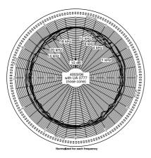
Fig. 7. Normalised directional characteristics of Types 4003 and 4006 with Nose Cone UA0777 fitted.
