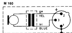
Positive pressure produces positive voltage on yellow cable lead (+)
